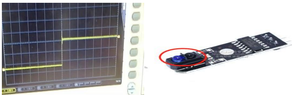
Figure 4&5. Infrared Detector. The blue light bulb will emit light, and the black light bulb will recycle it. The blue light bulb will emit light, and the black light bulb will receive it. If the black light bulb receives enough light, it will output a high voltage. If the black light bulb doesn't receive enough light, it will output a low voltage.
