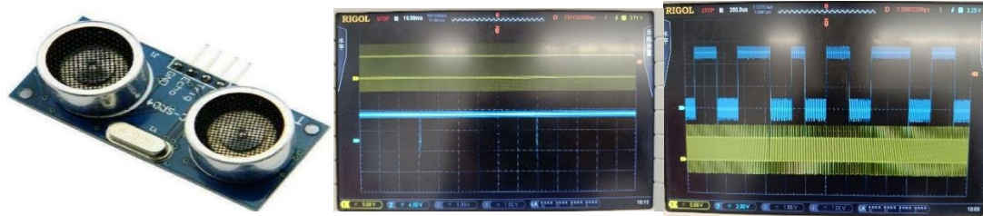
Figure 1&2&3. Ultrasonic Sensor. The right side (“Trig” shown as the yellow) emits an ultrasonic wave, and the left side (“Echo” shown as blue) recycles it. The right upper graph shows the voltage when the sensor is away from the obstacle, while the right lower shows the opposite situation.
